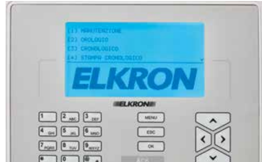
BLUE System under maintenance/ being programmed
